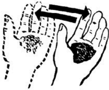
Dilatancy test: Shaking wet soil
