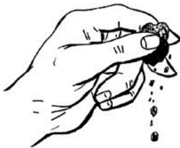
Dry strength test: Crumbling dry sample between fingers
